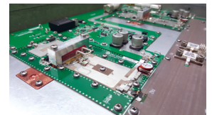
2 planar design RF pallets each of 1.7 kW
