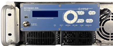
Up to 2 hot-swappable PSUs for AiO Series 1kW HR / 2kW 2 hot-swappable PSUs for AiO Series 3kW
